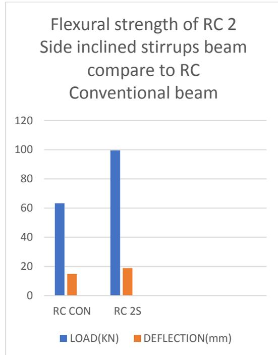
**4.2.2 Flexural Test for RC-2S beam:**
