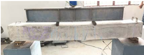
Fig 4.3 Flexure Beam B1
