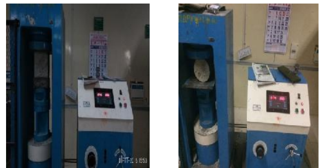
Fig.4 FLEXURAL STRENGTH OF PRISM
