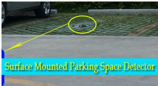
Fig.2 Surface mounted light dependent sensor
