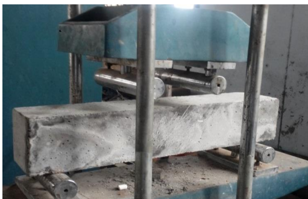
Fig.5 Experimental Setup for Flexural Strength Test
