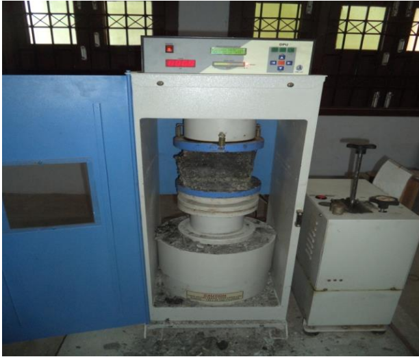
Fig.3 Experimental setup for Compressive strength test
