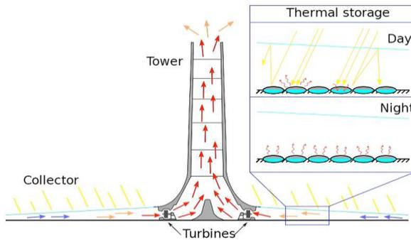
Fig: Schematic Diagram of solar updraft tower
