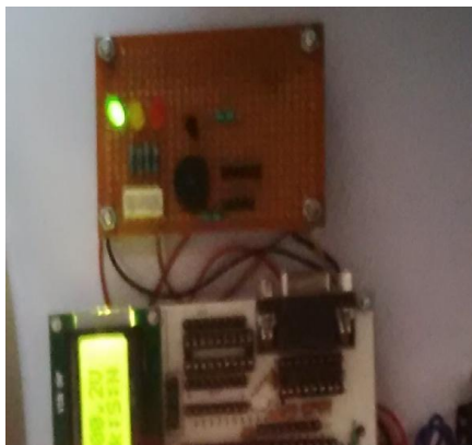
Figure 2.6 Green light indicates the applied load is below 4 Kg's.
