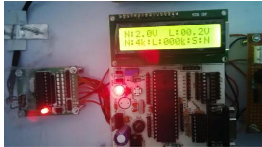
Figure 2.7 As the load reaches 4kgs. Red light indicator glows
