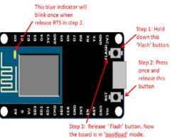
Fig 4.1 NodeMCU Board
