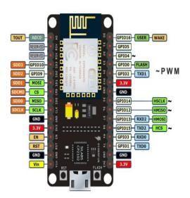
Fig 4.3 NodeMCU V3 Pinout
