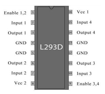
Fig 5.1 L293D Motor Driver Circuit
