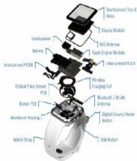
Figure 4. Expanded view of Apple watch
