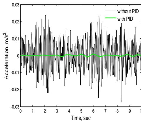
Fig 8. Random Input – PID Wheel acceleration
