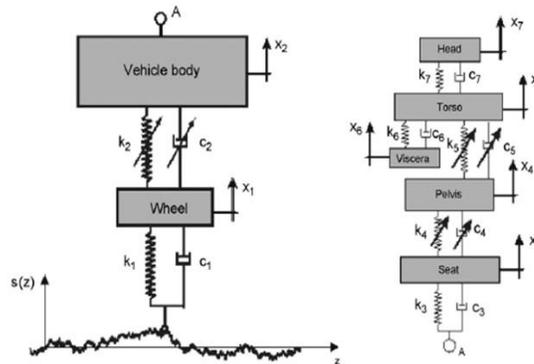
Fig 1. Quarter Car Model -Biodynamic Model
