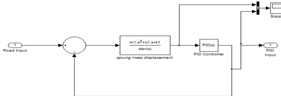
Fig 5. Simulink PID Controller of a Quarter Car Model
