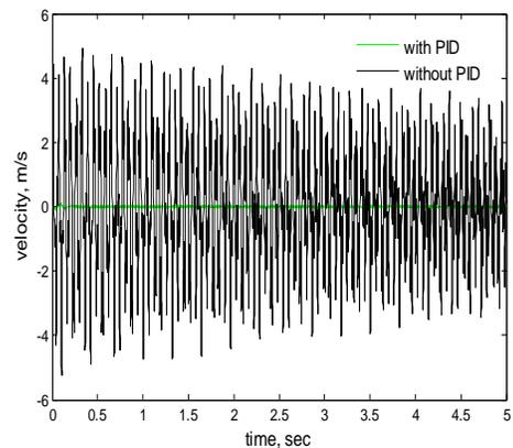
Fig 16. Sinusoidal Input - Half Car - PID Pitch Velocity
