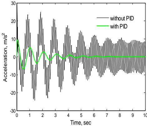
Fig 13.Sinusoidal Input - PID Torso acceleration
