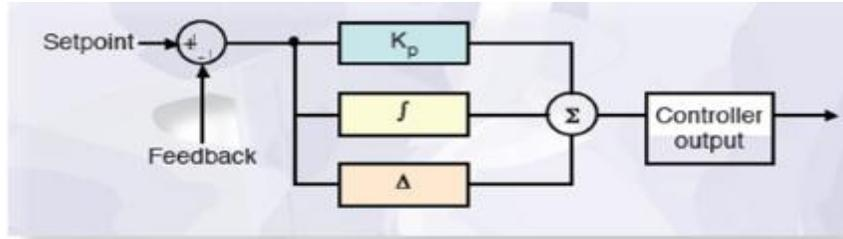
Fig 4. PID Controller
