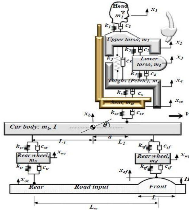
Fig 2. Half car coupled to Human body
