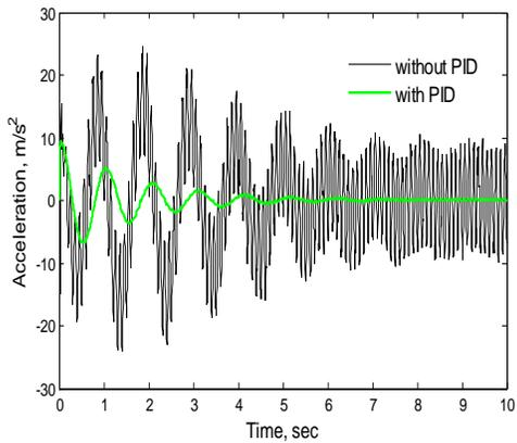
Fig 12. Sinusoidal Input – PID Pelvis acceleration
