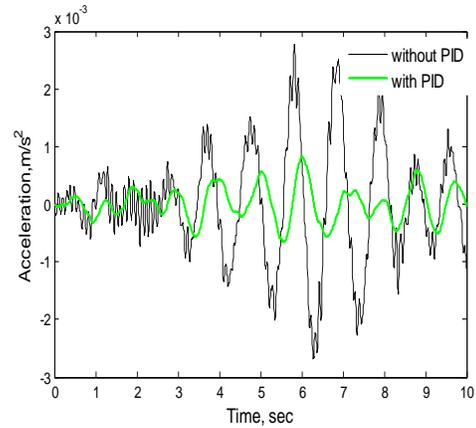
Fig 10. Random Input – PID Vehicle Body acceleration
