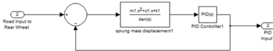
Fig 6. Simulink PID Controller for Half Car Model
