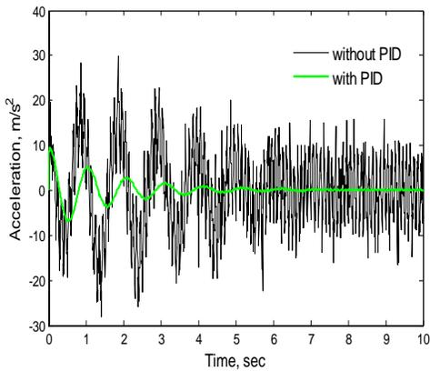
Fig 11. Sinusoidal Input – PID Seat acceleration
