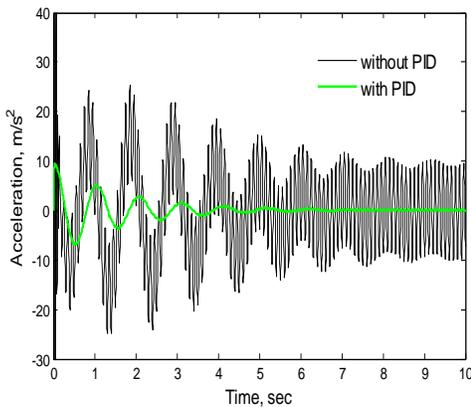
Fig 15.Sinusoidal Input - PID Head acceleration
