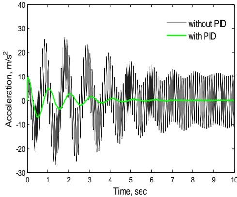
Fig 9. Sinusoidal Input - PID Vehicle Body acceleration
