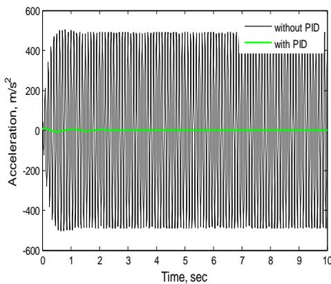
Fig 7. Sinusoidal Input - PID Wheel acceleration
