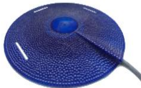
Fig III: Seat Pad Accelerometer
