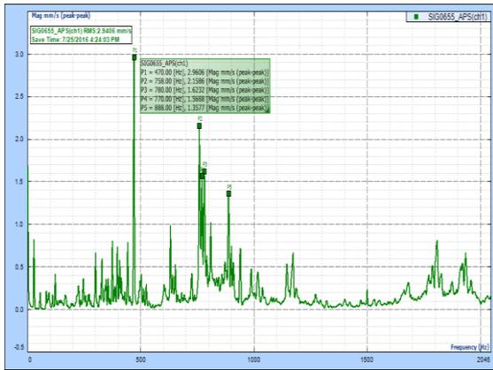
Fig. 4 Frequency spectrum at top of the DC Motor
