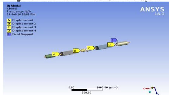
Fig. 10 Boundary Conditions of Motor Generator System
