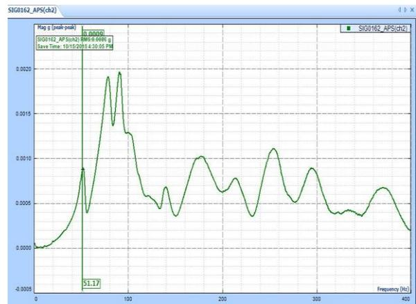
Fig. 8 Frequency spectrum at top of the DC Motor
