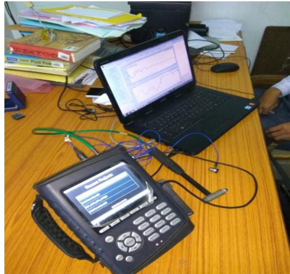
Fig. 7 Photograph of instruments, hardware and software used for Natural Frequency Test (NFT) on motor generator system
