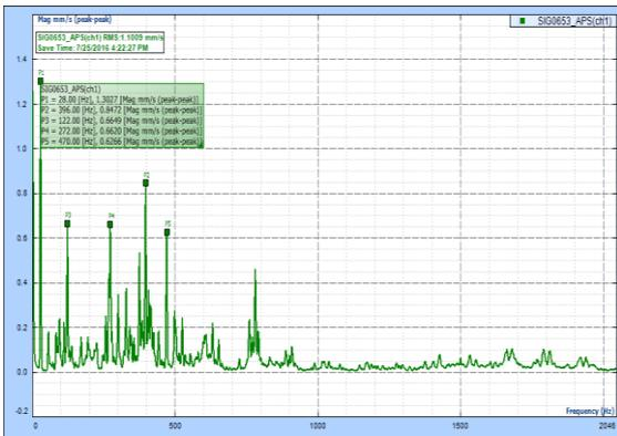
Fig. 5 Frequency spectrum at top of the frame
