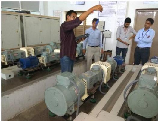
Fig. 1 Noise measurement taking at of D C motor by using FFT analyzer and Condenser micro phone
