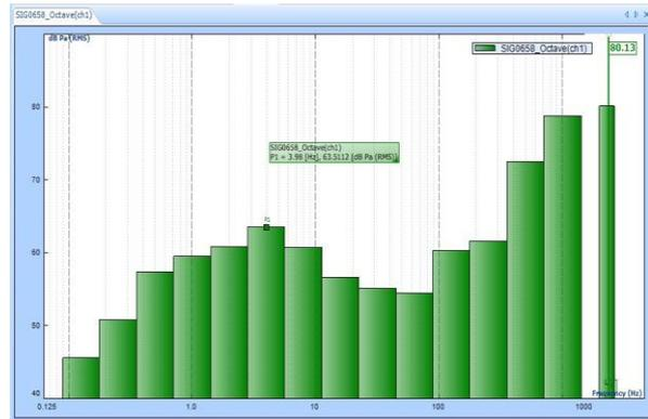
Fig. 2 Noise Spectrum at the top of the Motor Generator System
