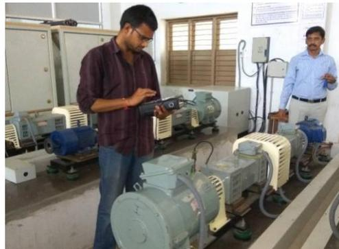
Fig. 3 Vibrtion measurement at the D. C motor using FFT analyzer and piezo electric sensor
