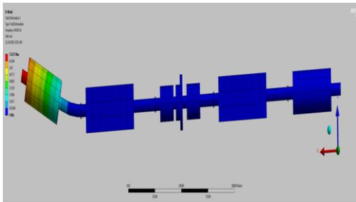
**Fig. 11** First mode of Motor Generator System
