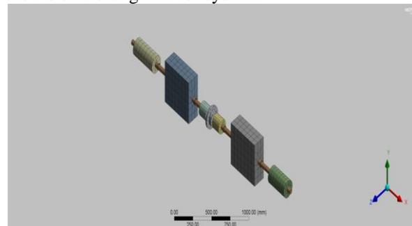
Fig. 9 Meshed Model of Motor Generator System
