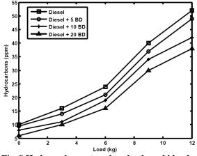
Fig. 8 Hydrocarbons at various loads and blends (d) Nitrogen Oxide: With the increase in % of biodiesel, NO<sub>x</sub> is increased which is due to generation of higher exhaust temperatures and also due to lower cetane number.
