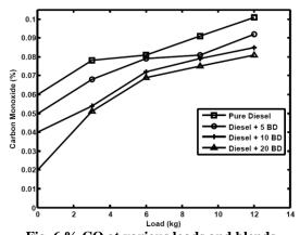
Fig. 6 % CO at various loads and blends(b) % of CO<sub>2</sub>: It decreases with the % increase in biodiesel due to better combustion.
