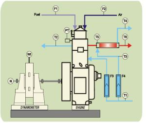
Fig.2 Schematic of Test Setup
