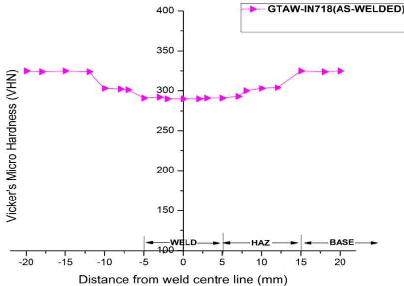
Fig 6 Vickers Micro-hardness survey of IN718 GTA welds
