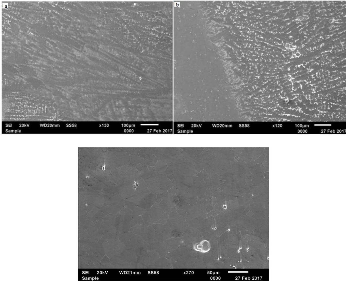
Fig 5 SEM microstructure of IN718 GTA welds (a) Fusion zone and (b) Weld interface and (c). Base Metal
