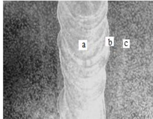
Fig 3 Optical Macrostructure of IN718 GTA welds
