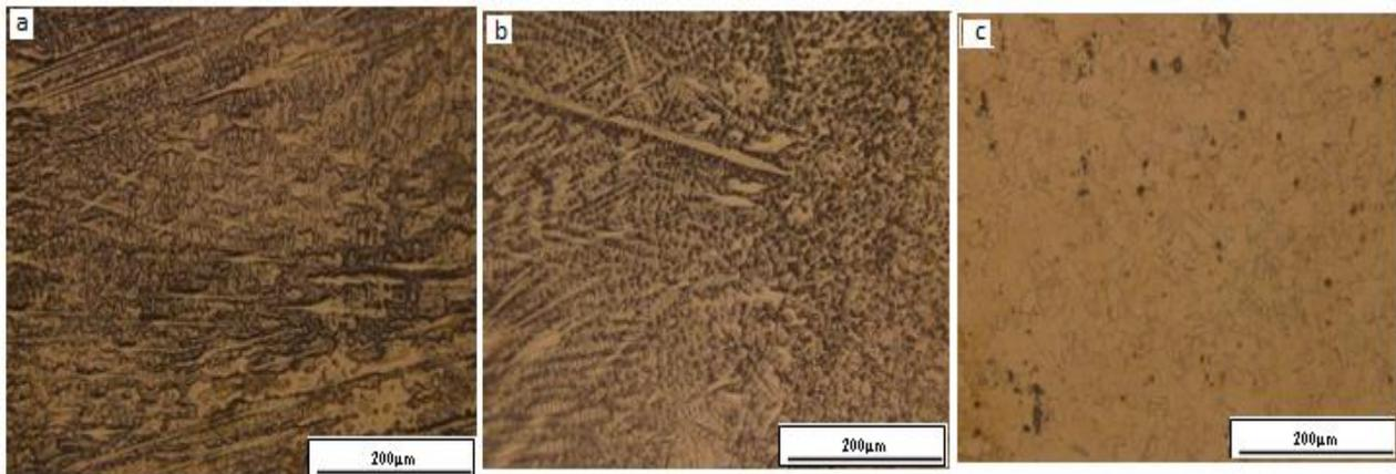
Fig 4 Optical microstructure of IN718 GTA weld (a). Fusion Zone (b). Weld Interface and (c). Base Metal
