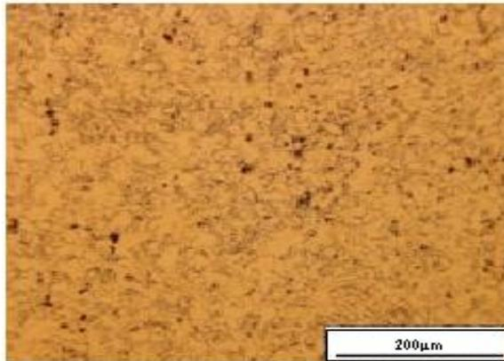
Fig 2 Optical Microstructure of IN718 alloy
