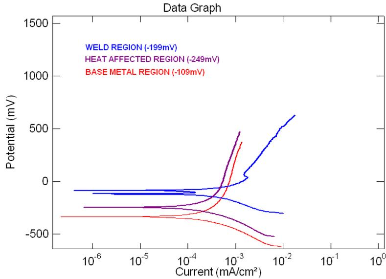
Fig 7 Potentio-dynamic polarization curves of IN718 GTA welds
