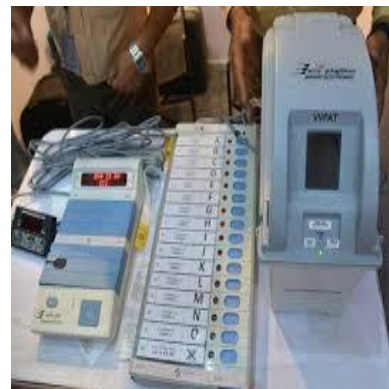
Figure 1. Electronic Voting Machine (Source: www.indiatvnews.com)
