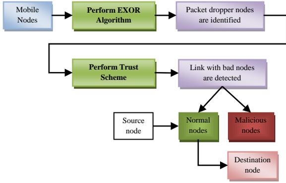
Fig.2. Block diagram of proposed algorithm
