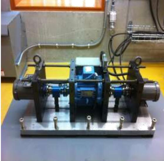
**Figure 1.1 Load sharing motor test bench used for the practical observations.**
