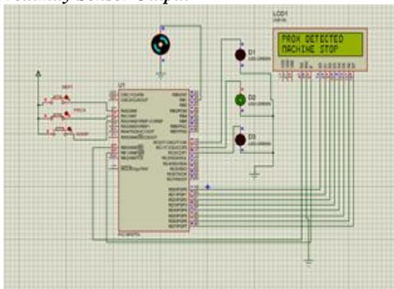
**Figure 6 Proximity Sensor Output.**
