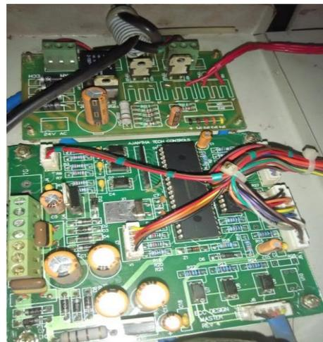
**Fig. 3. Power loom Control**
