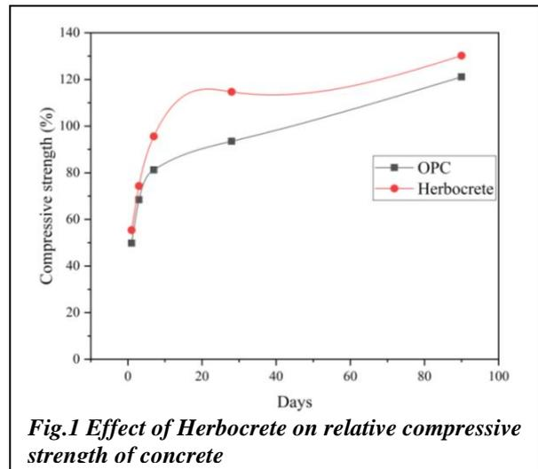
Fig.1 Effect of Herbocrete on relative compressive strength of concrete
