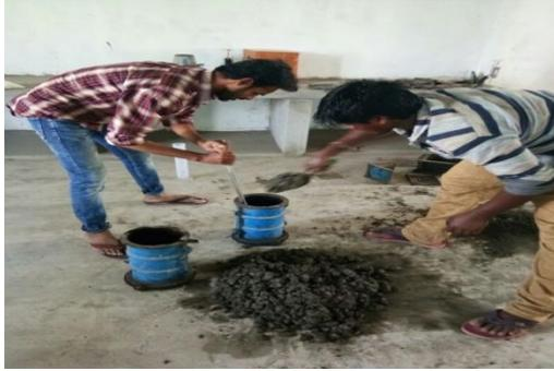
Fig3. Cylinders casting
