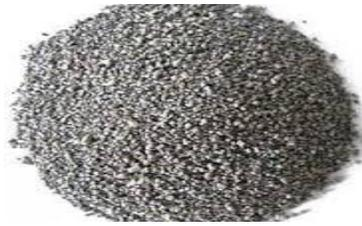
Green sands are typically black, or gray, not green. Chemically bonded sand is typically a medium tan or off-white color. Figs. 1.1 & 1.2 show the unprocessed foundry sand and green sand respectively.
