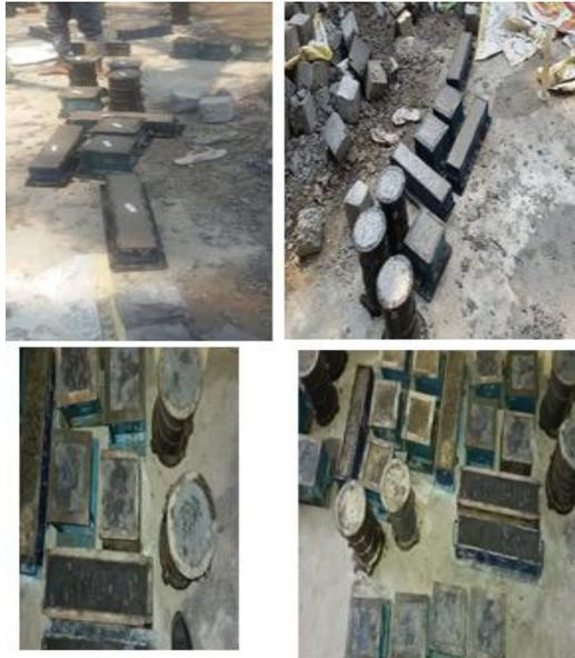
Figure 8.4: Pictures shows the Casted specimens
