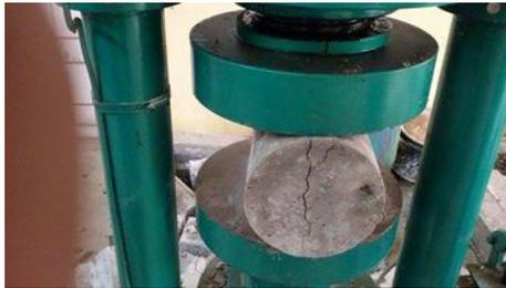
Figure 8.3: Picture shows the Split tensile strength
