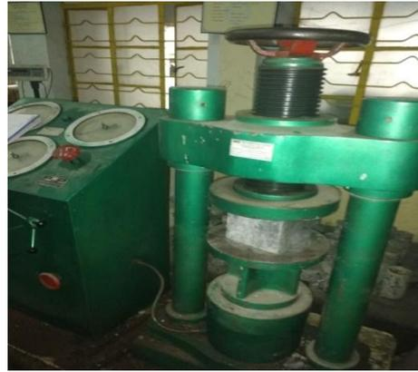
Figure 8.1: Picture showing the compressive testing for cubes
