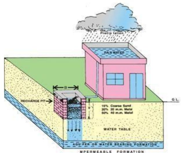
**Fig1.existing method of Rain water harvesting**
