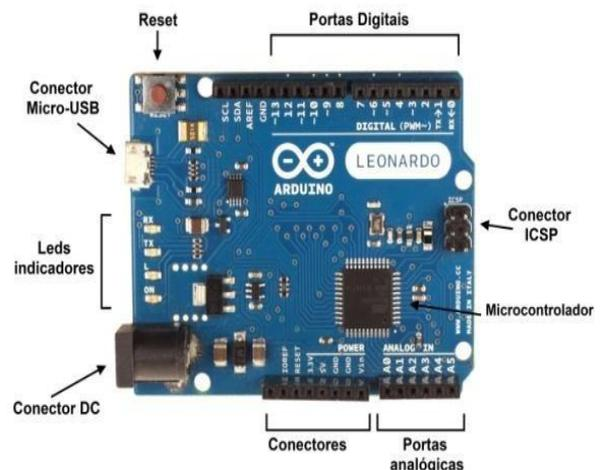
Figure 2.Arduino and its parts
