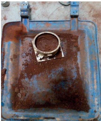
Figure 1.a: Standard proctor compactor
