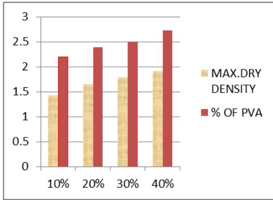
Figure 1: Max. dry density for varying % of PVA
