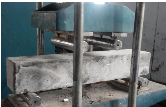
Fig.5 Experimental Setup for Flexural Strength Test
