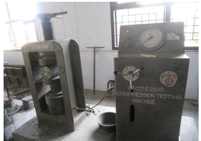
Fig.4 Experimental Setup for Split Tensile Strength Test
