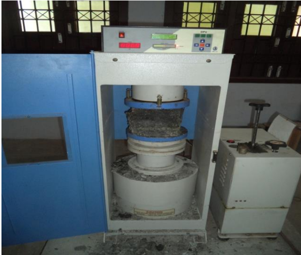
Fig.3 Experimental setup for Compressive strength test
