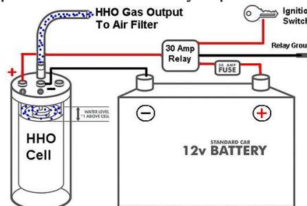
Fig 3: Hydrogen Generator
