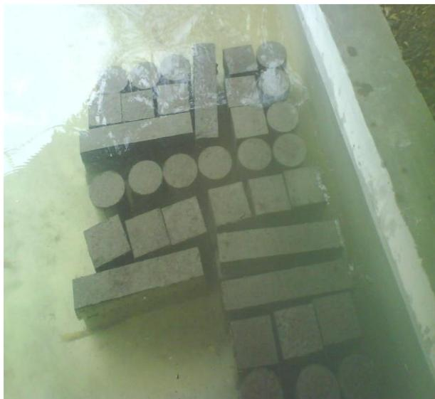
Fig. 4.3: Curing of concrete specimens
