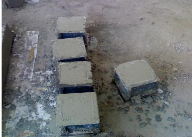
Fig. 4.2: Casting of concrete specimens
