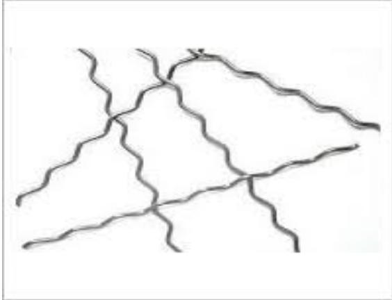
Fig. 2.2: Steel fibers
