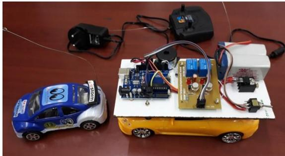
The output of the alcohol sensor is in the analog nature which should be converted into digital format. This is done by the analog to digital converter of the microcontroller unit. The microcontroller controls the entire circuit. When the measured value reaches the threshold (here it is 255) the microcontroller switches the ignition ON. Then relay cuts off automatically and buzzer produces sound.
