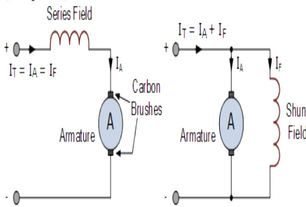
Fig 6.1 Series and Shunt Connected DC Motor
