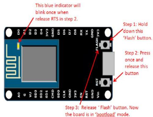
**Fig 4.1 NodeMCU Board**
