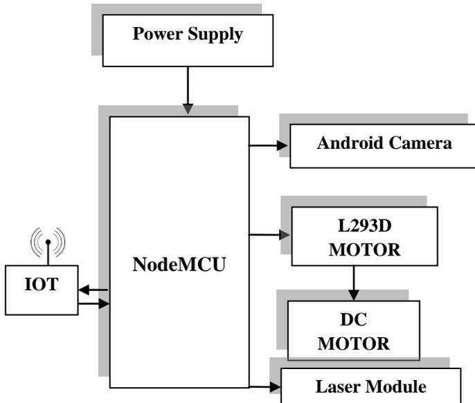
Fig 1.1 ROBOT Section
