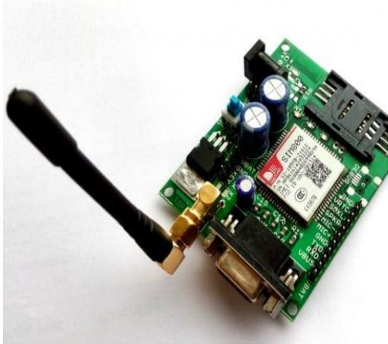
Figure 5: GSM SIM800
