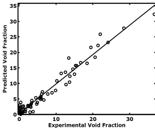
Fig. 3 Pariplot of Experimental Void Fraction Vs Predicted Void Fraction of Ann
