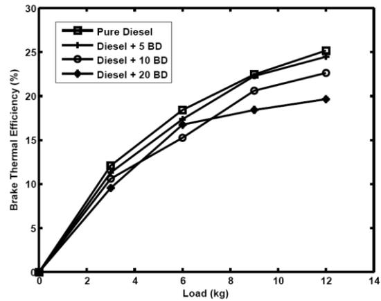
**Fig. 3 Brake Thermal Efficiency at various loads and blends**
