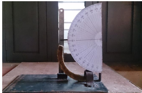
Fig 3:Set up for hygric strain measurement
