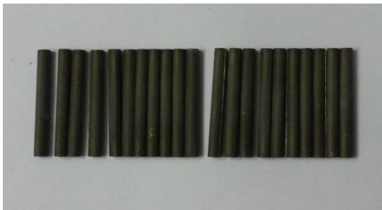
Fig 4: \text{Cr}_3\text{C}_2 - NiCr Coated Ti6Al4V Specimens
