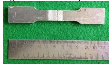
Fig-9.1 Tensile specimen made as per ATSM-E8
