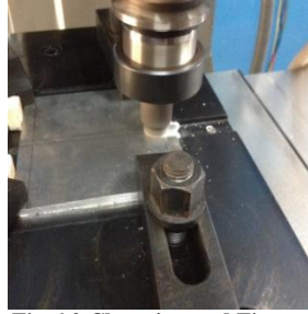
Fig-6.2 Clamping and Fixture setup performing FSW
