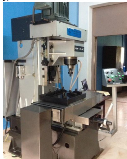
Fig-5 The friction stir welding machine
