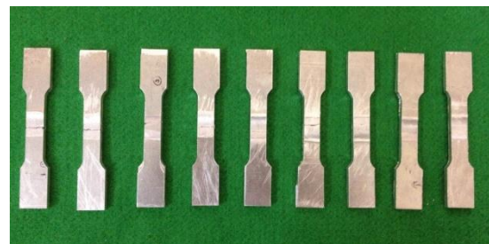
Fig-9.2 Tensile specimens of all different passes
