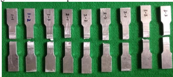
Fig-11 Failure of tensile specimens of AA5083 with the addition of TiB 2
