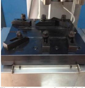
Fig-6.1 Fixture used to hold the base materials
