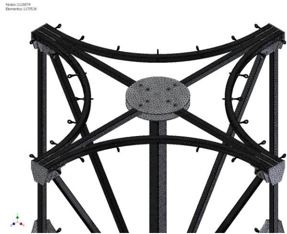
Fig. 4 Meshing of the structure
