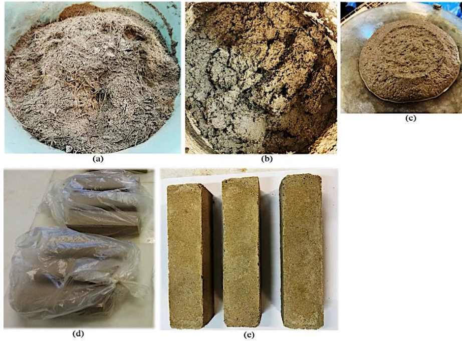
Fig. 2 Production of CSF-reinforced one-part AMMO samples: (a) Preparation of dry mix, (b) Fresh AMMO, (c) Flow table test, (d) Pre-curing of the samples, and (e) Samples after the curing period.
