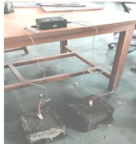
Fig. 3 CP-CMM with Concrete Cubes
