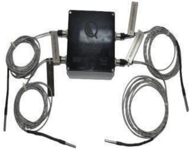
Fig. 1 C-Probe's Concrete Maturity Meter System
