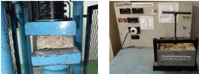
(a) Compressive testing (b) Thermal conductivity testing Fig. 4 Testing of the sample for the compressive test and thermal conductivity
