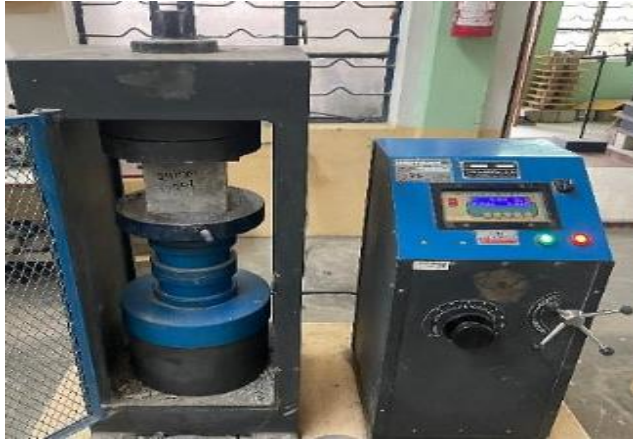
Fig. 5 CTM used for cube testing
