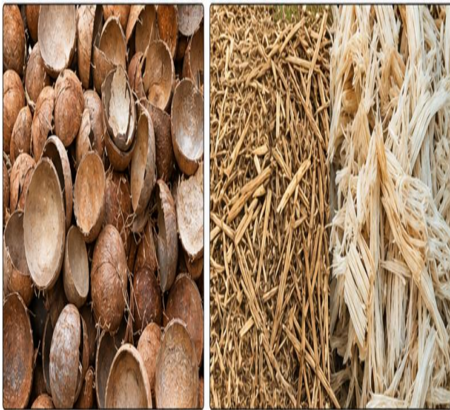
Fig. 2 Preparation of coconut shell and sugarcane agro-waste for aggregate substitution
