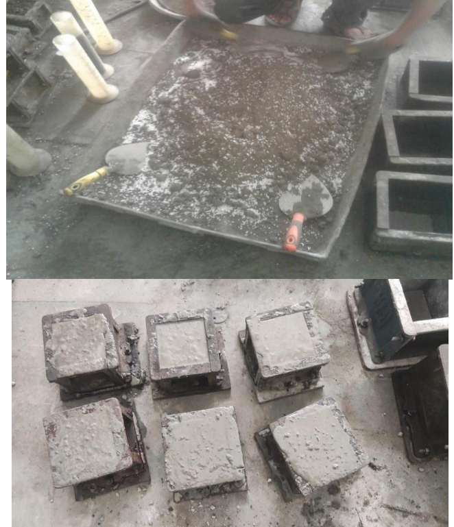
Fig. 3 Concrete batching and mould filling operations
