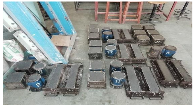
Fig. 4 Cast cube specimens and application of wax curing membrane
