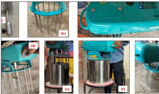
Fig. 4 Rheometer setup employed to assess the rheological characteristics of fresh MSWI-1 mix
