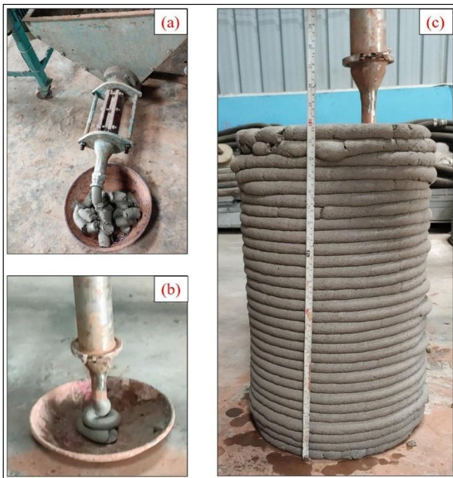
Fig. 8 Printability assessment of (a) Mix MSWI-2, (b) Mix MSWI-1, and (c) 3D printed structure using MSWI-1 mix.
