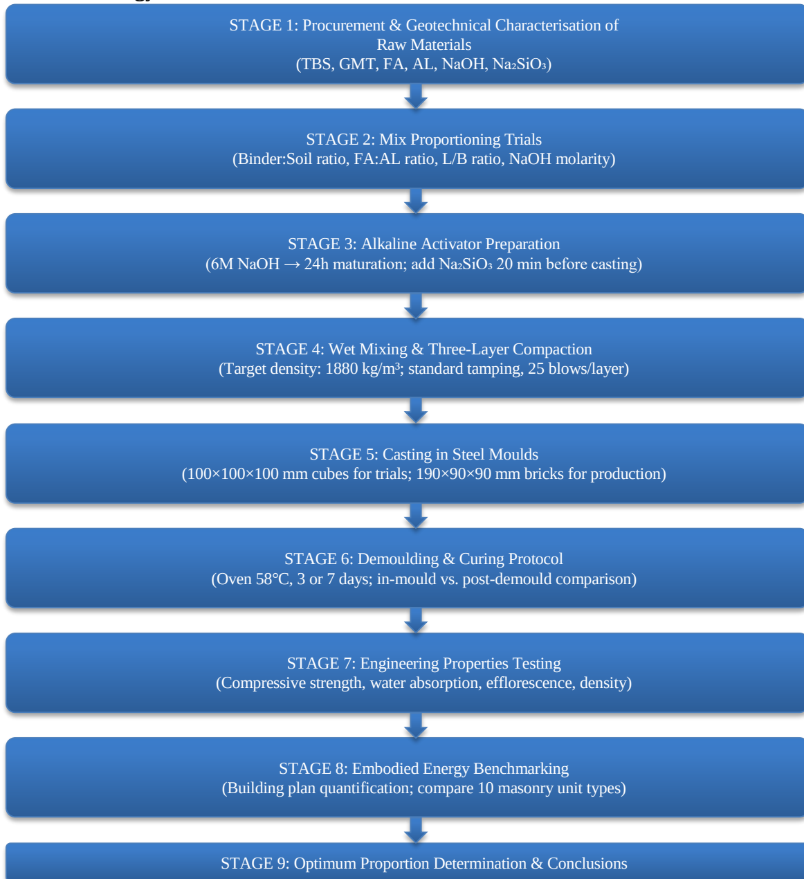
Fig. 10 Experimental methodology flowchart for GSEB production and evaluation
