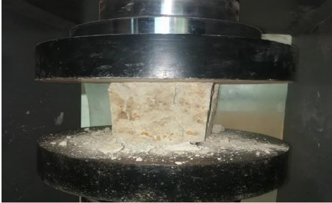
Fig. 7 Compressive strength testing of blocks
