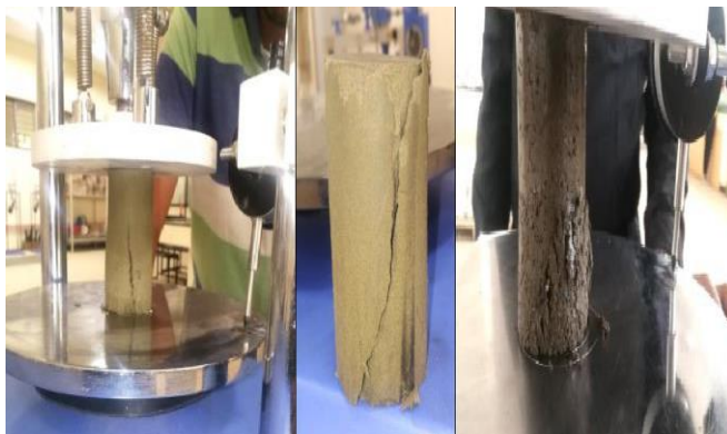
Fig. 4 Unconfined compression test equipment and its different failure specimens
