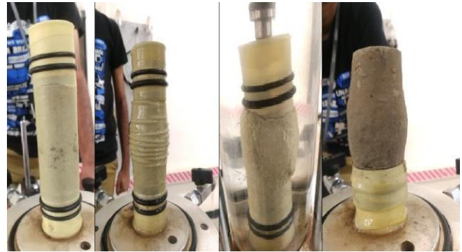
Fig. 5 Triaxial compression test specimens before and after compression process
