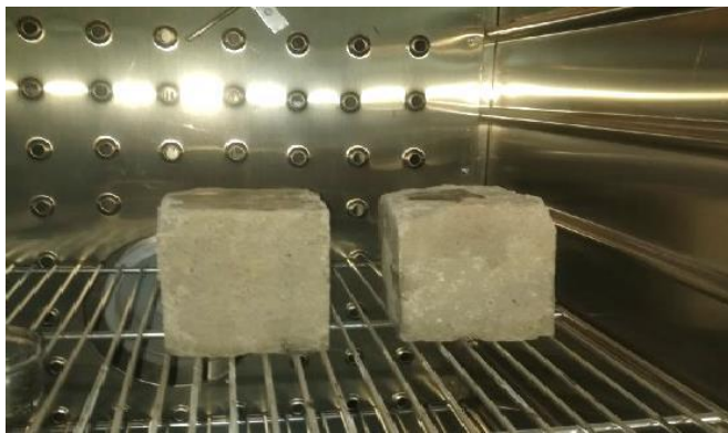
Fig. 8 Blocks N1 & N2 cured in oven at 58°C
