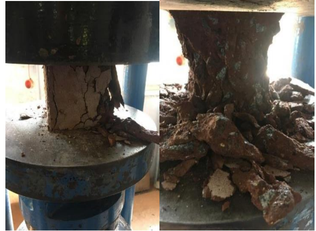
Fig. 8 Concrete specimen after testing
