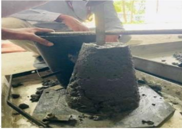
Fig. 7 Slump Test of Fresh Concrete
