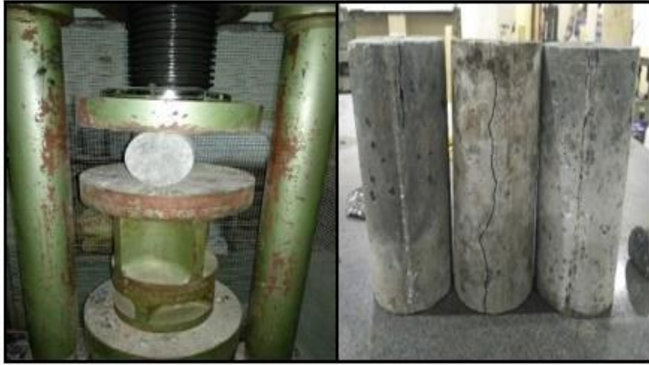
Fig. 10 Split tensile strength test setup
