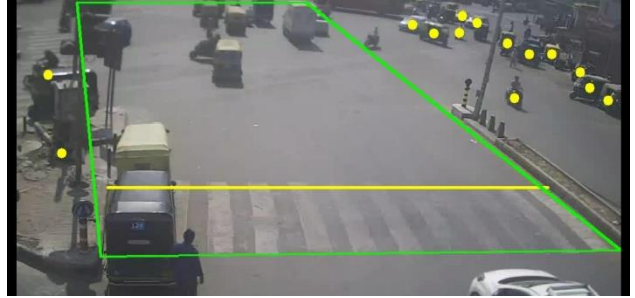
Fig. 3 CCTV video 2 ROI and wrong side detection line
