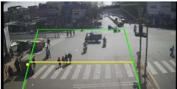
Fig. 2 CCTV video 1 ROI and wrong side detection line
