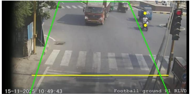
Fig. 5 CCTV video 4 ROI and wrong side detection line
