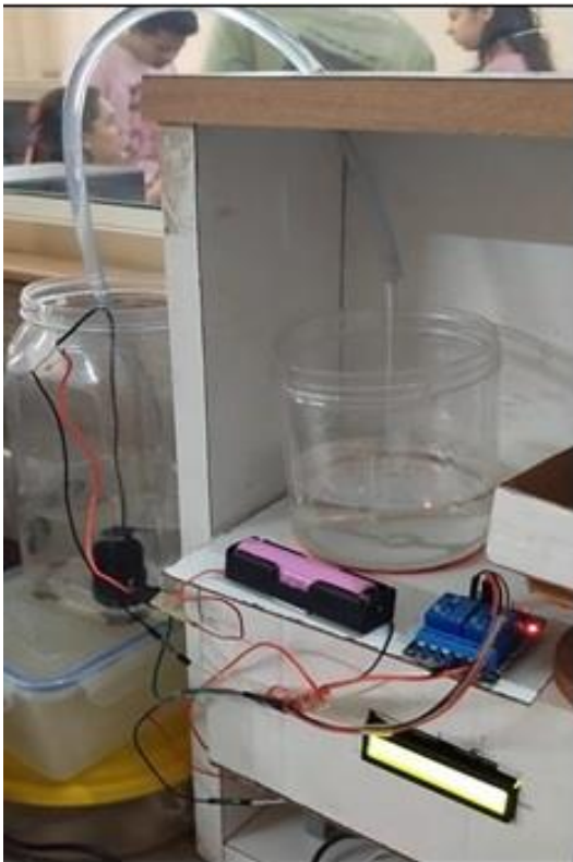
Fig. 9 Liquid dispensing system
