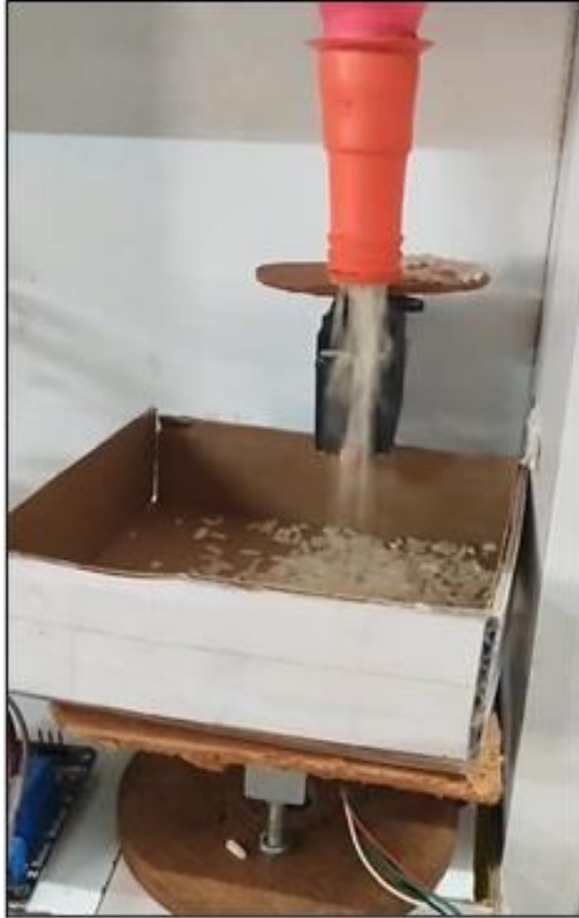
Fig. 8 Grain dispensing system
