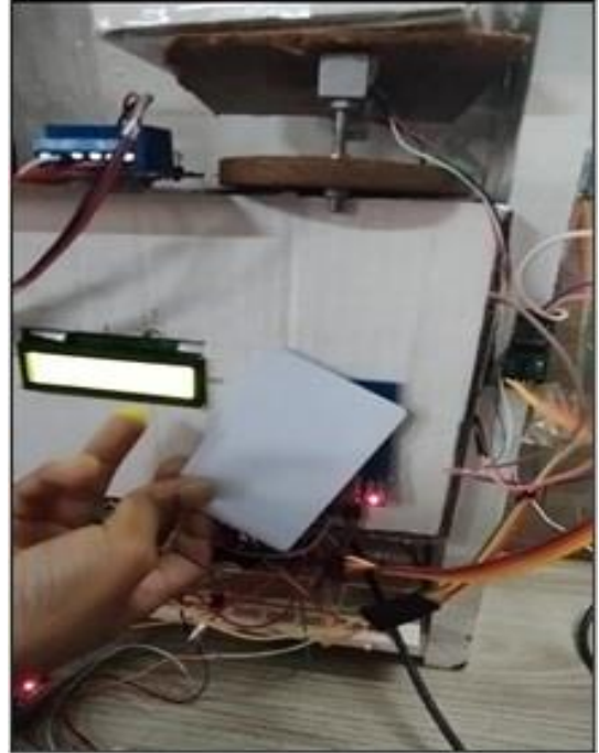
Fig. 10 Authentication system using an RFID card
