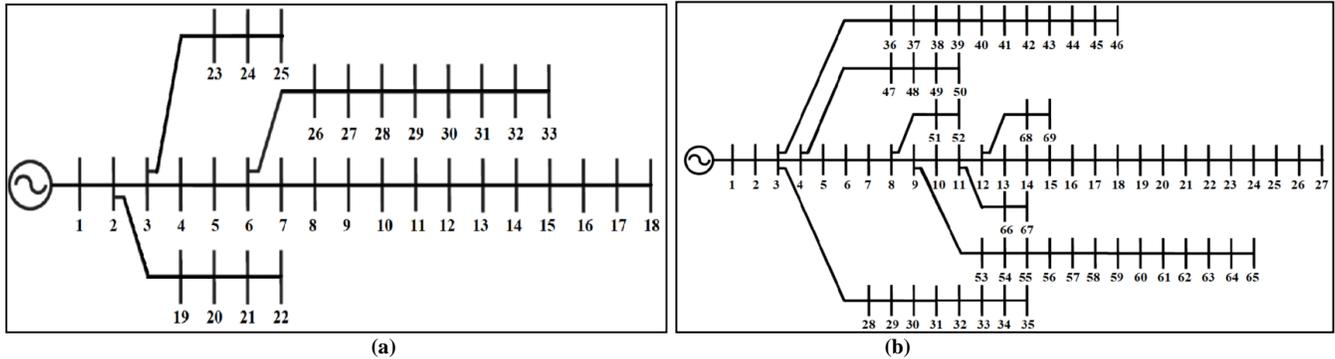
Fig. 1 Single line diagram, (a) IEEE 33-bus system, and (b) IEEE 69-bus system.
