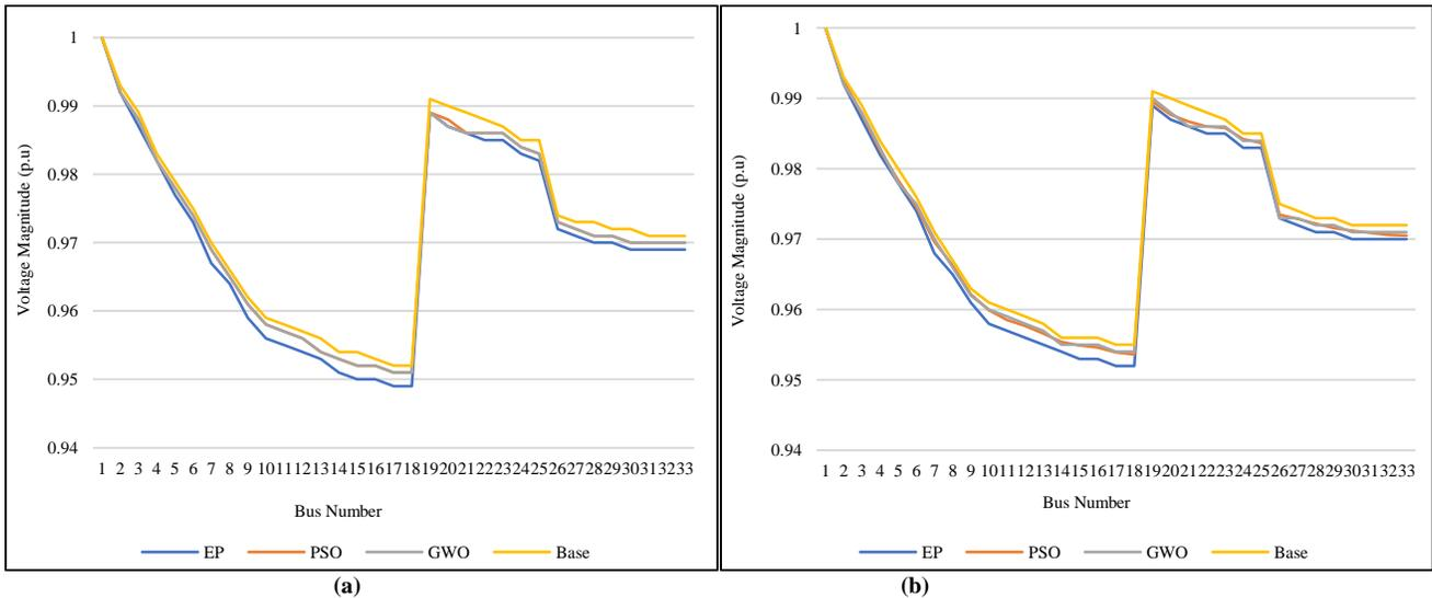
Fig. 3 Network voltage profile within the 33-bus system, (a) Without PV integration, and (b) With PV integration on weak buses.
