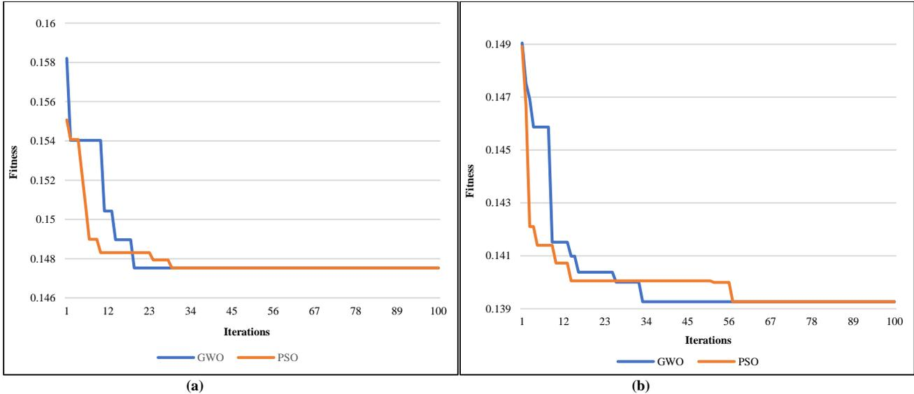
Fig. 2 Convergence curve for minimizing power losses in the IEEE 33-bus system, (a) Without PV integration, and (b) With PV integration.
