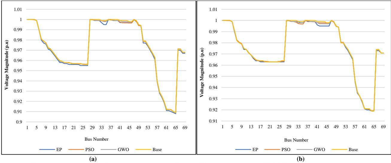
Fig. 4 Network voltage profile for 69-bus system, (a) Without PV integration, and (b) With PV integration on week busses.
