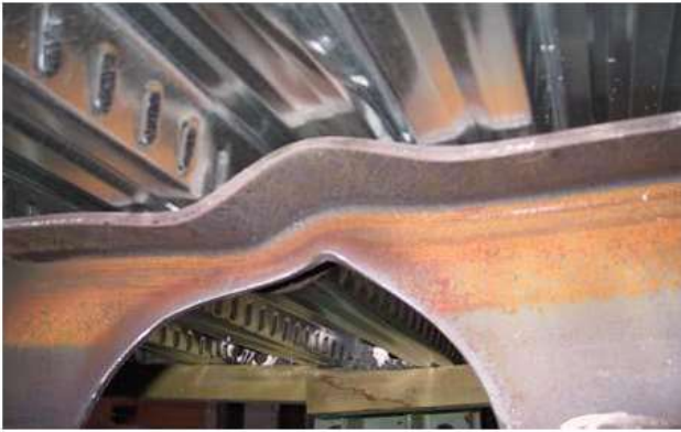
Fig. 8 The Mechanism of Vierendeel [48]
