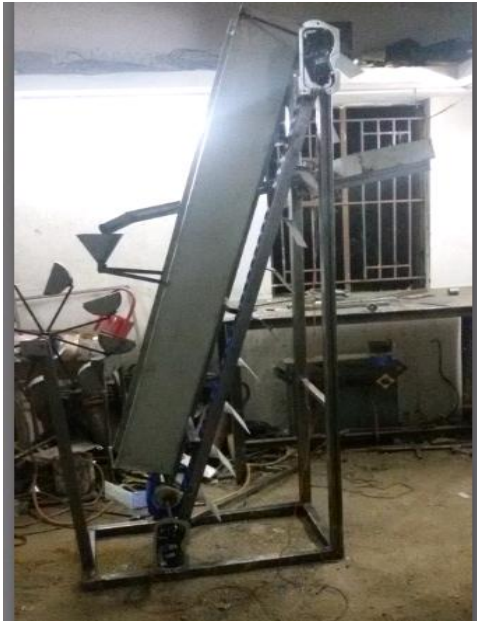
(1.7 a) Side view of Fabricated Reusable Sand power Generator
