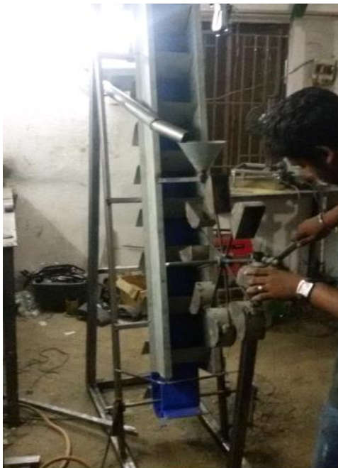
(1.7 b) Front view of Fabricated Reusable Sand power Generator
