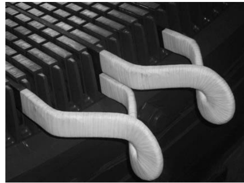
Fig-3: Stator winding inside stator core slot.
