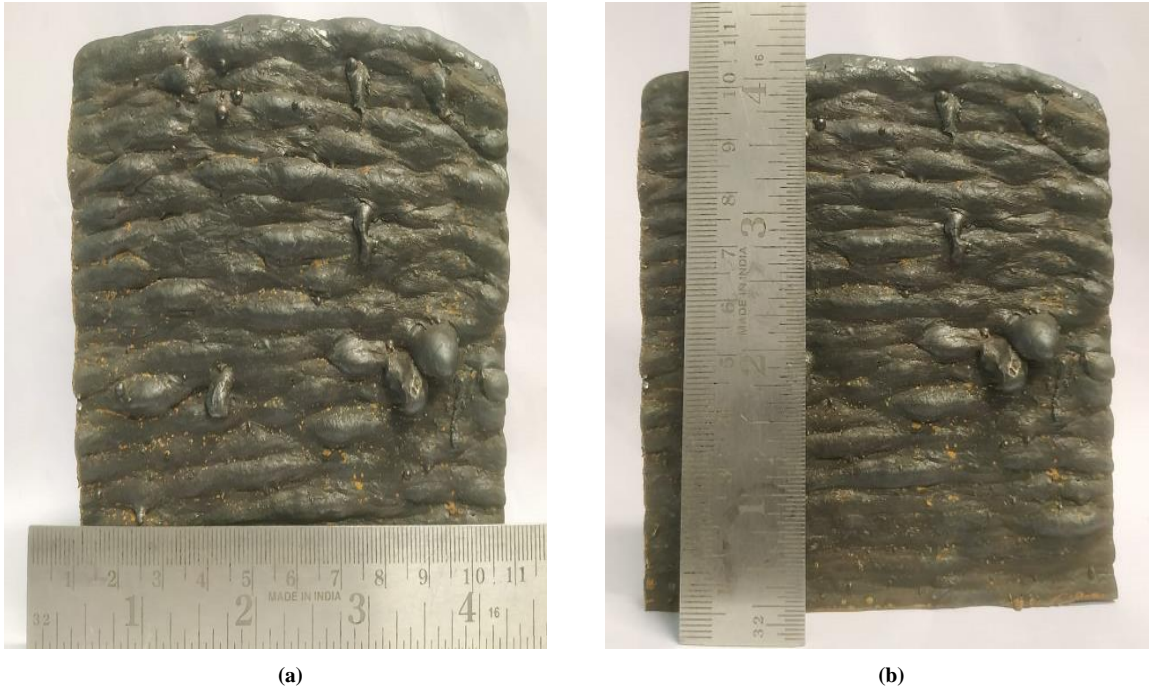
Fig. 32 Multilayer structure (a) Length, and (b) Width obtained in experimental work for the optimized input parameters.
